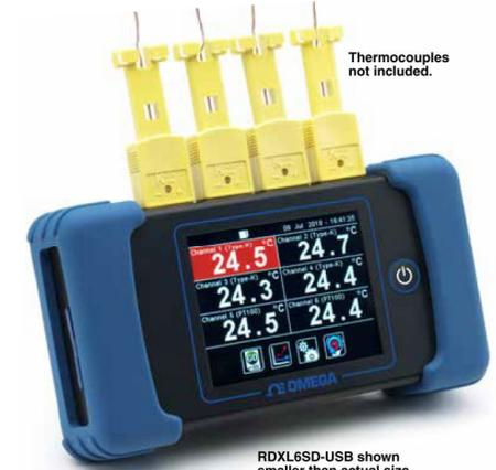
The RDXL6SD-USB is a six-channel touch screen data logger that accepts four thermocouple and two RTD inputs. Each channel has individually configurable HI/LO alarms. The intuitive touch screen interface allows each channel to be configured separately for input type, math, alarm and display options. All six channels can be displayed and logged simultaneously or individually. Data can be logged as fast as once a second and is stored on the included 4 GB SD card in Excel® compatible format.
